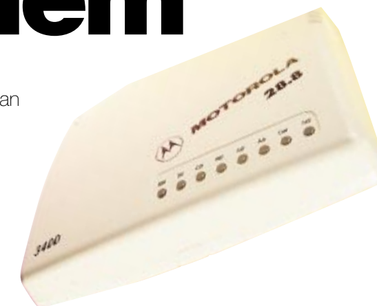
V34 28.8kb/sec modem or one of the new V34 Plus 33.6kb/sec modems.
